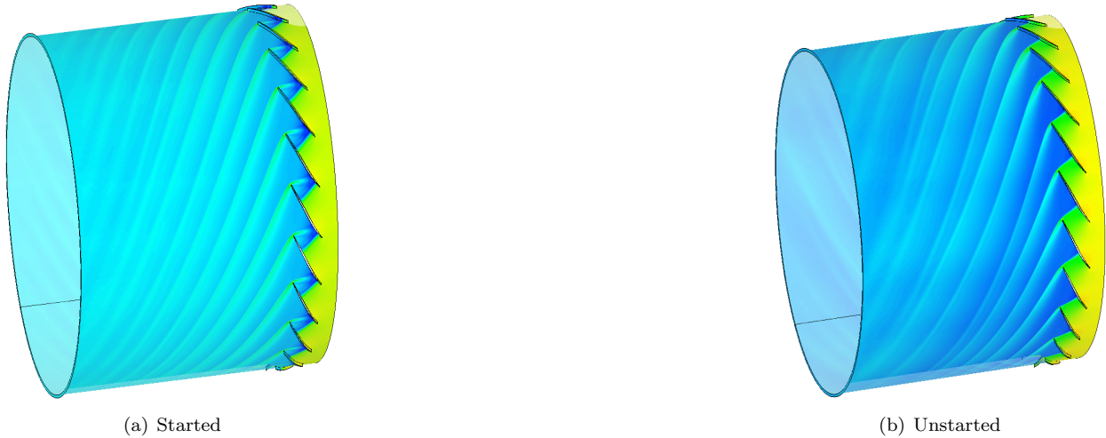
Figure 1. A 2-D full annulus simulation with stagger variation in blades to predict MPT generation. (a) started fan, and (b) unstarted fan.
