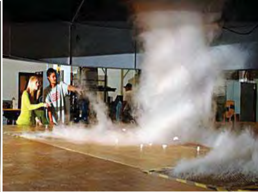
The world largest moving Tornado/Microburst Simulator D_{\text{tornado}} = 0.5\text{m} \sim 1.5\text{m}
