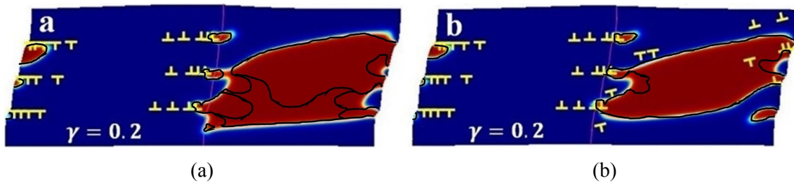
Fig. 3 Stationary solutions for interaction of the phase transformation to a HPP (red color) and dislocations in a bicrystalline sample subjected to normal stress and shear strain, without (a) and with (b) plasticity in the right grain. Dislocation pileup causes PT at pressure (averaged over the grain) significantly smaller than under hydrostatic loading with a single dislocation. Dislocations promote PT by producing stress-tensor concentrators (a) but also suppress PT through relaxation of stresses near the tip of the dislocation pileup (b). The contour lines of the equilibrium PT work are presented in black and, in most cases, coincide with the stationary phase interfaces. This figure is reproduced with permission from Ref. 39).
