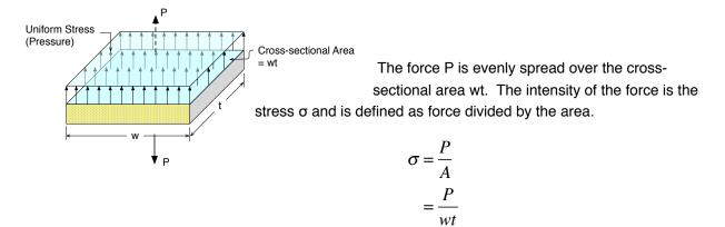
The stress is normal, meaning perpendicular, to the cross-sectional area and is often designated as a "normal stress." Typical units are:
