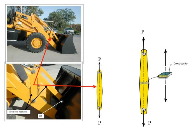
The force P acts on a typical cross-section shown on the right.
