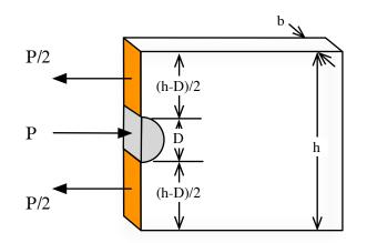
It is imperative that a FBD be drawn that cuts through the candidate failure surfaces. The areas and the forces acting on the surfaces are used to calculate the stresses.
