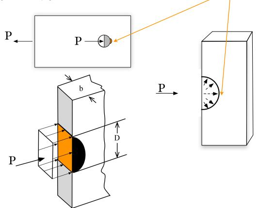
A practical approach has historically been taken to characterize this type of problem. The bearing stress is calculated using the **bearing area** that is a rectangular patch size D by b. It is assumed that the bearing stresses are uniformly distributed over this area.
