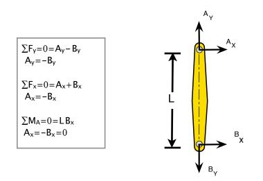
Note: A two force member has **no moment** applied at any location on the member, otherwise the two horizontal forces would not be zero.
