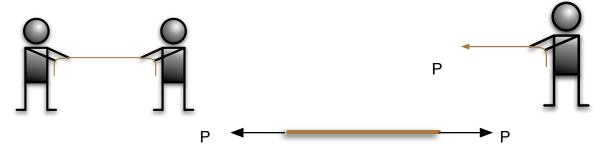
P is referred to as an axial force. Only two forces are required to keep the rope in equilibrium. The two forces in the Free Body Diagram, FBD, are collinear. A FBD of a member with two frictionless pins is used to prove that only two equal and opposite forces are required to satisfy equilibrium.
