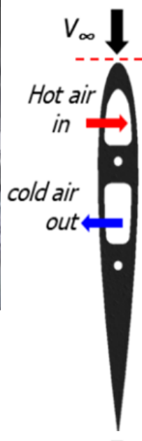
• Ice accretion on Inlet-Guild-Vanes (IGV)
